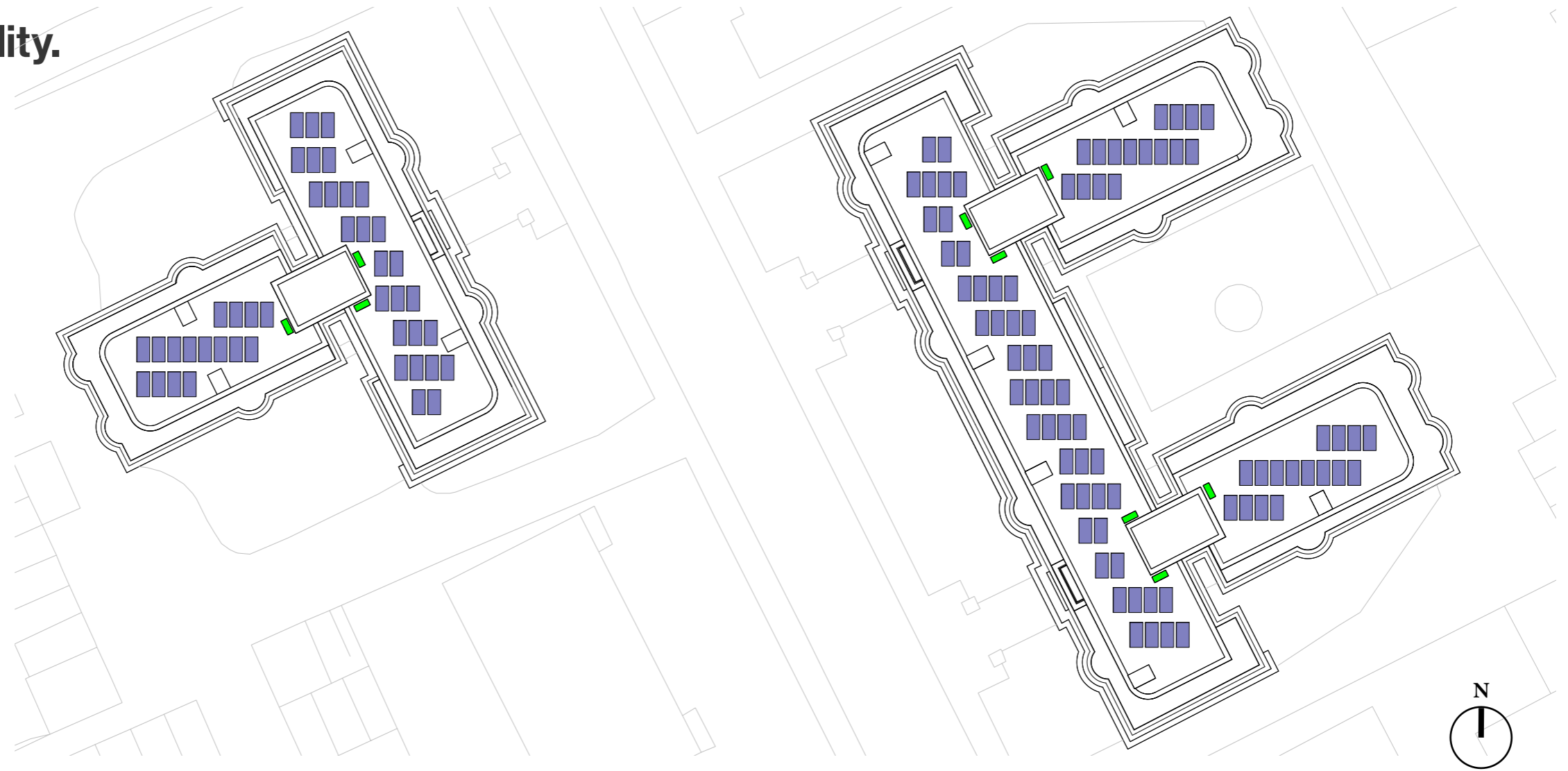
Proposed photovoltaic panels and heat pumps.
